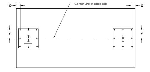
Mark the locations of the pilot holes. Drill the pilot holes to the size recommended by the table top manufacturer. Install the screws through the mounting plate into the table top.
