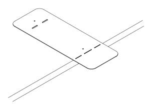
FORM THE MOUNTING PLATE BRACKET Use a straight edge to bend the smaller lip along the perforated lines.
